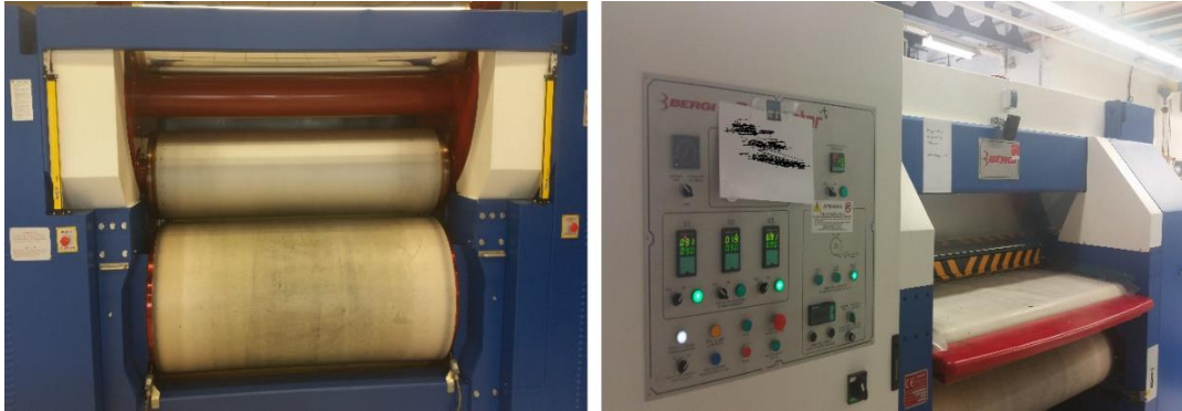
Figure 3. 6- Embossing machine (back View on the left and Front View on the right)
