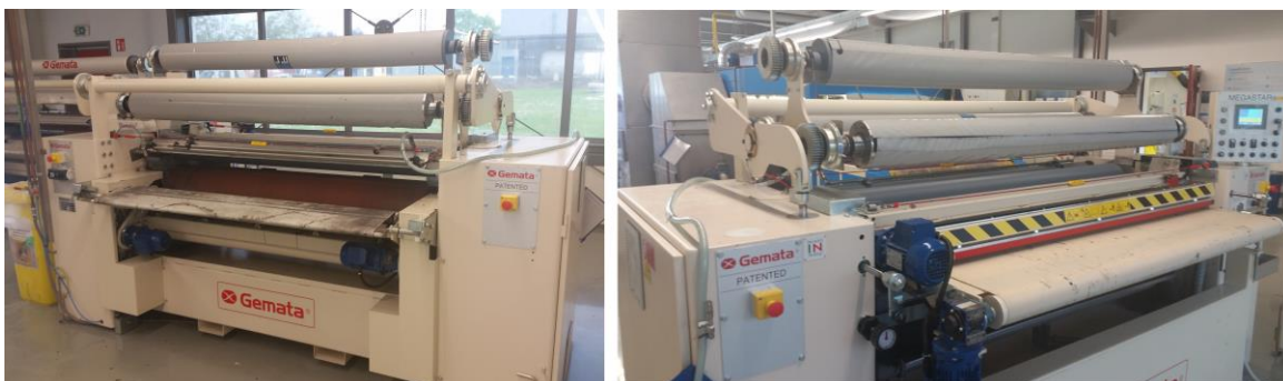
Figure 3. 5- Roller Coater (Back View on the left and Front View on the right)
