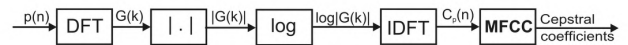
Fig. 4. A schematic diagram of the classical algorithm for determination of MFCC coefficients.
