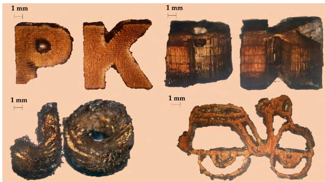
Figure 10. Cationic photopolymerization of glycidyle: DGEBA/EPXPROP (70%/30% w/w) in the presence of biphenyls derivatives/Iod (0.2/2% w/w) for 3D printing.
