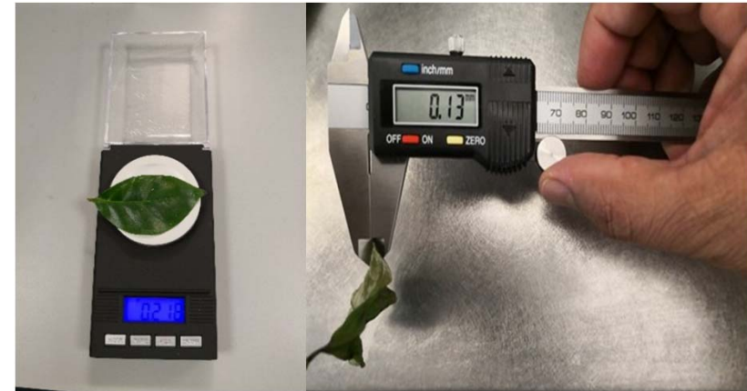
Fig. 3: Demonstration of Measuring the weight and thickness of leaves using digital scale and Vernier calliper respectively
