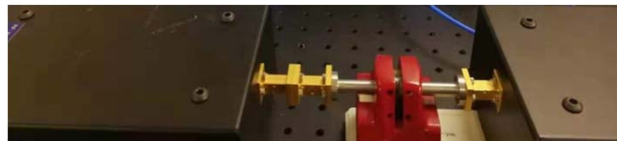
Reference signal: measured by connecting the two halves of the corrugated waveguides of the MCK without sample between them together.
