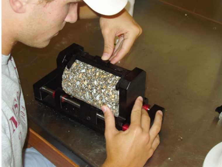
Figure 3.8 Attaching Studs to Specimen Using Jig
