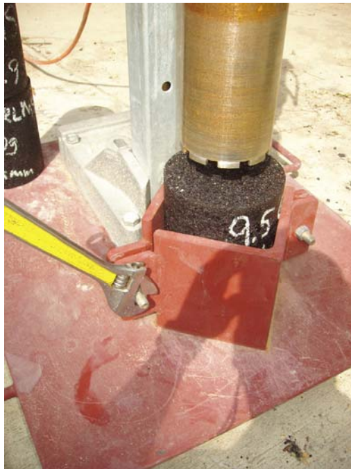
Figure 3.1. Preparing to Core Compacted Sample to Produce Dynamic Modulus Test Specimen
