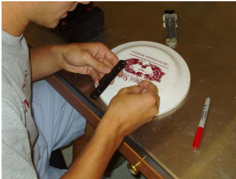
Figure 3.7 Placing epoxy on Studs
