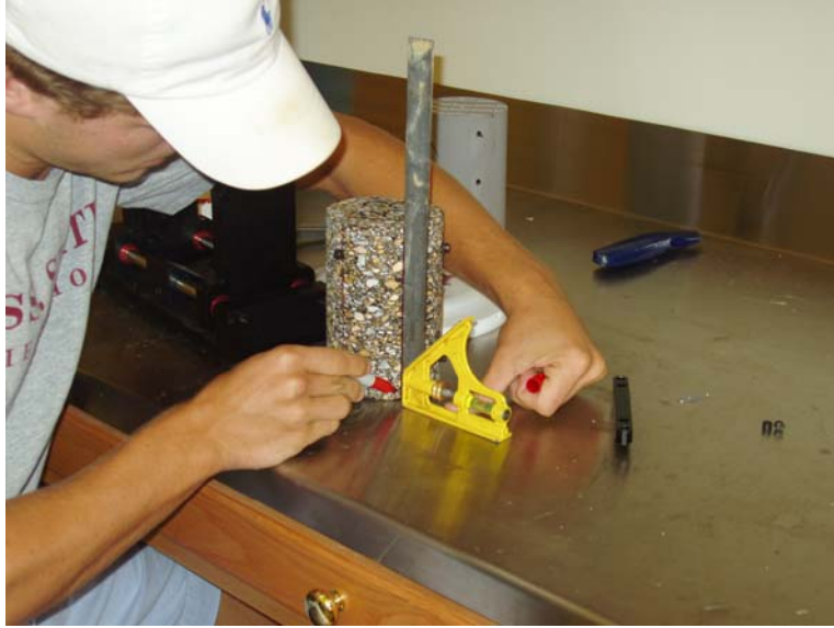
Figure 3.6 Marking Reference Lines
