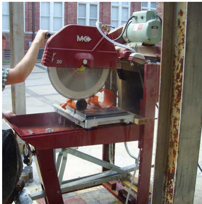
Figure 3.4. Sawing End of Dynamic Modulus Test Specimen
