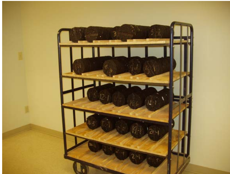
Figure 3.11 Prepared APA Specimens
