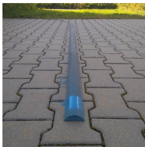
Figure 3. Portable measuring FBG sensor.
