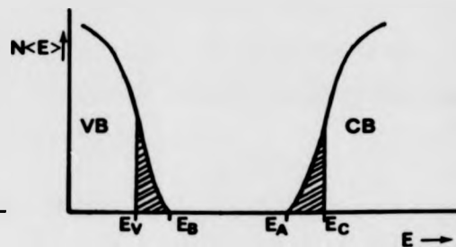
Fig. 2F - Electron density of states curve for an "ideal" non-crystalline solid showing tailing of localized states at band edges according to Mott's suggestion.
