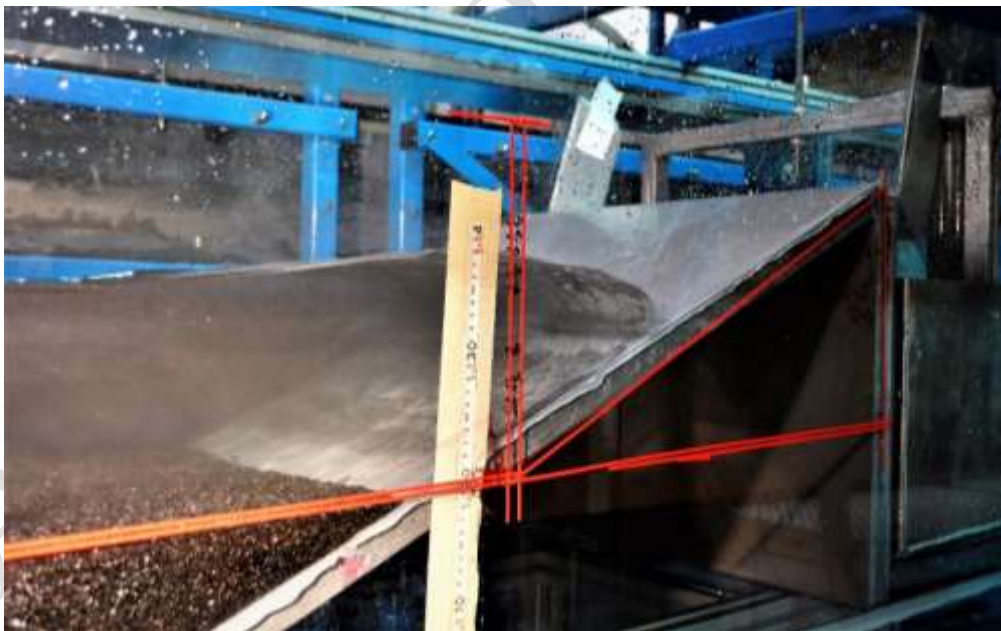
698 Fig. 1. Experimental set-up a. Cross-section along the length of wave channel, b. The overtopping 699 measurement techniques and location of wave gauges (A-A'), c. Photograph of an experiment with 700 shingle foreshore d_{50} of 13 mm
