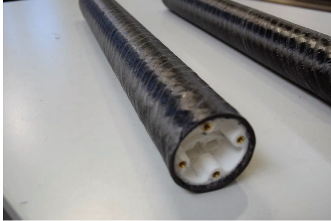
Figure 9. Fabricated CPV with AM-fabricated end-cap with integrated pressure reducer.
