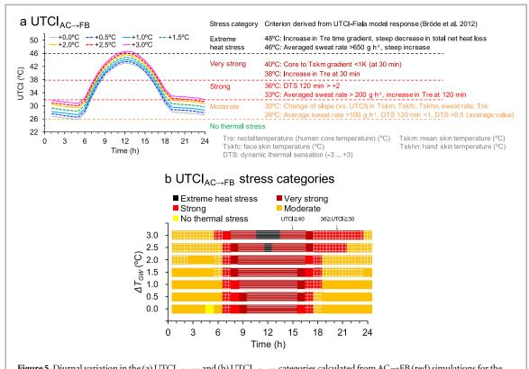
**Figure 5.** Diurnal variation in the (a) UTCI<sub>AC $\rightarrow$ FB</sub> and (b) UTCI<sub>AC $\rightarrow$ FB</sub> categories calculated from AC $\rightarrow$ FB (red) simulations for the current and six future climates simulated with  $\Delta T_{GW}$  for residential areas (figure 1d). For WBGT see supplemental material.
