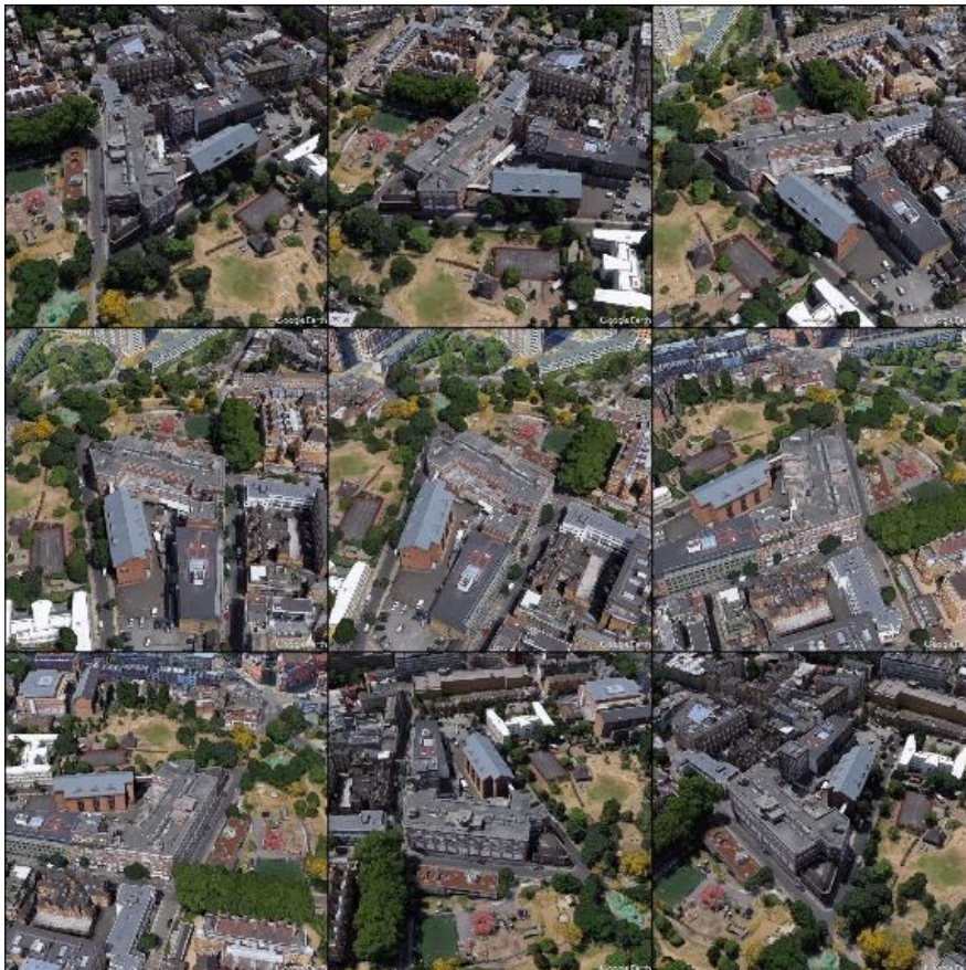
Figure B-2. Nine sample images captured by Google Earth using a pre-programmed Google Earth “tour”. Images are used to create a dense point cloud “tile” in Agisoft PhotoScan Professional (Figure B-3).
