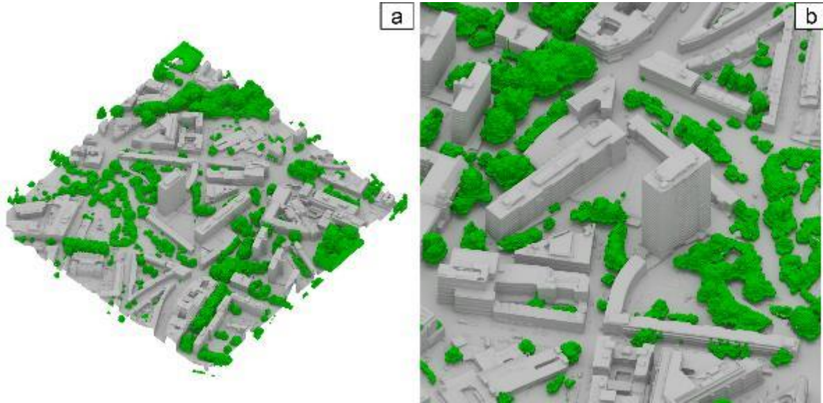
Figure B-1. Urban surface geometry includes a vector-based 3D surface model (grey) and voxel-based model of vegetation canopy elements (green). The central London (UK) study area rendered using Blender (Blender, 2018) showing: (a) full extent (450 m x 450 m) and (b) more detail around the centre of the area.
