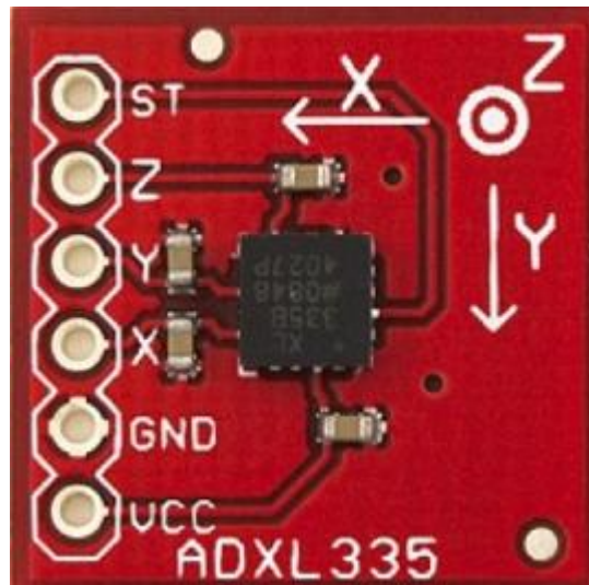
Figure 3-5 A typical 3-axis accelerometer breakout board (Hobby Electronics, 2018)
