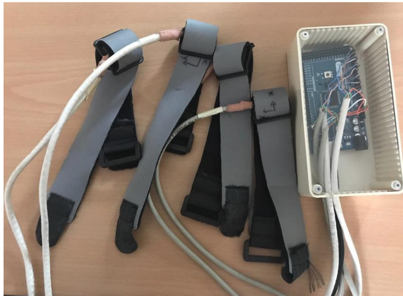
Figure 7-6 Photo of the accelerometers and microcontroller housed in suitable casings
