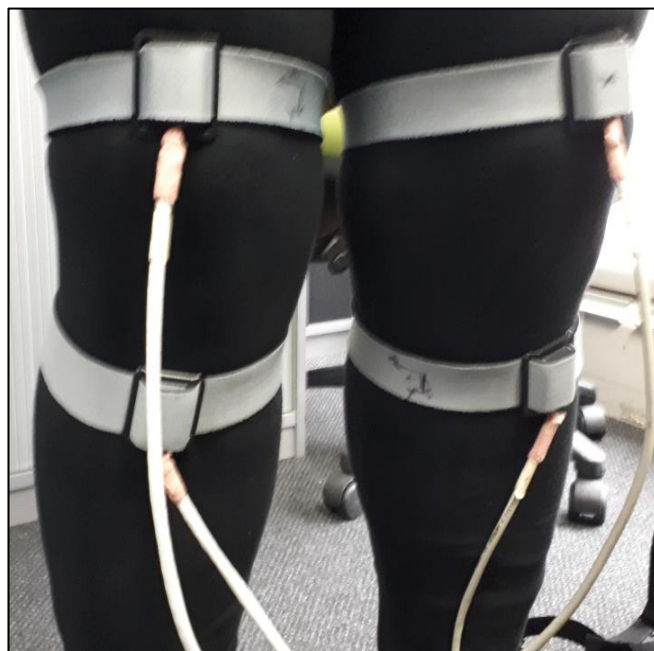
Figure 7-8 Accelerometers strapped to the thighs and shanks of an adult subject
