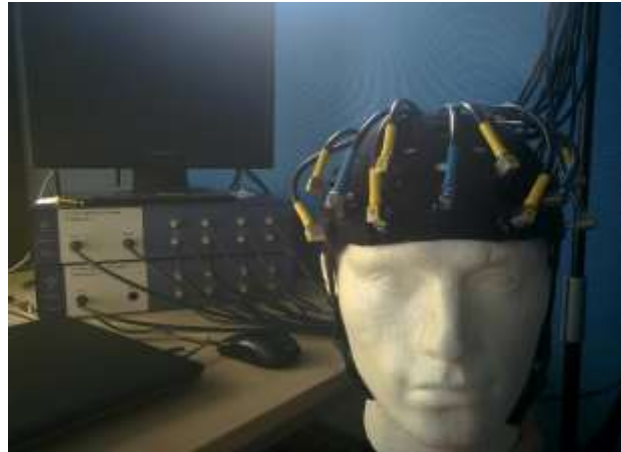
Figure 3.3 Montage of the 12-channels functional Near-Infrared Spectroscopy. Receivers are in blue, transmitters in yellow.
