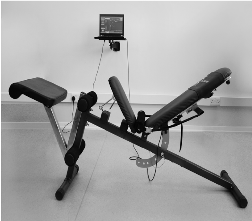
Figure 1 Abdominal test and evaluation systems tool (ABTEST version 3) device used for the evaluation of abdominal strength.
