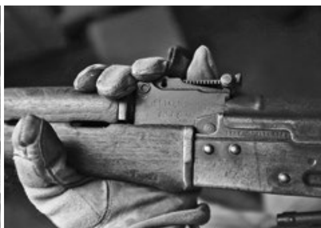
Markings on the fire selector of a Chinese-manufactured AK47 Type 56 variant (l.) and Arabic markings on the receiver of an Egyptian-manufactured AK47 pattern rifle (r.). An effective SALW marking, registration and record-keeping goes a long way in securing stockpiles and preventing diversion, laying the ground work for a broader tracing or tracking programme.
