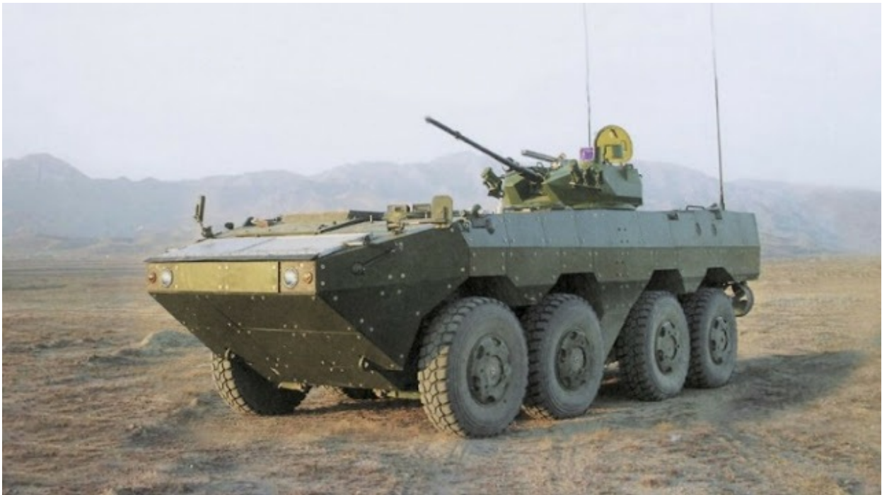
Image Attribute: VN1 APC - in this photograph fitted with a 30 mm autocannon in a turret. In 2015, Argentina ordered 110 Chinese VN1 APCs. The VN1 is an 8x8 wheeled and amphibious armored fighting vehicle, which is an export version of the ZBL-09 APC operated by the Chinese army. The Argentinan version is destined to be armed with a 12.7
