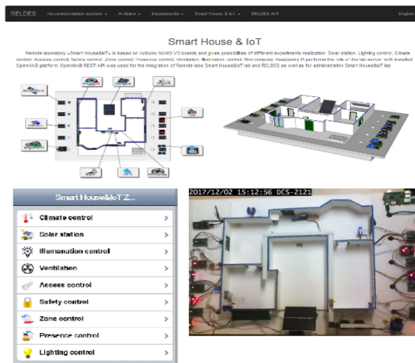
Fig. 8. Remote Lab Smart House & IoT web-interface
