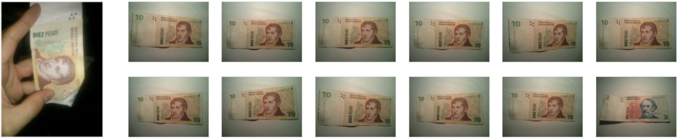
Figure 19: Bank note recognition example. 11 samples of each denomination were used to train. A new image (showed in the first column) is queried, obtaining the image list sorted by similarity on the right. There are enough elements on the top of the list that vote for the same class. Therefore, there is a majority consensus and the result: “10 pesos”.
