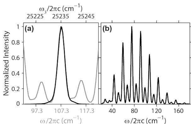
Fig. 4. Narrowband probe and fs/ps RCARS spectra. (a)  $N_2$  RCARS spectrum (gray trace, lower gray x-axis) taken with probe after fundamental spectral filtering but before SFG grating filtering. Grating filtered  $\Delta\nu = 3.0 \text{ cm}^{-1}$  probe spectrum (black trace, upper black x-axis). (b) Spectrum of 7.8 atm of  $N_2$  at room temperature, probed at 8 ps delay (transitions out of rotational states  $J = [2, 20]$ ) by probe from (a).
