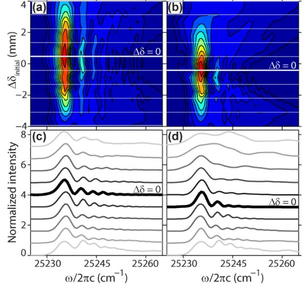
Fig. 3. Opposite chirp matching without (a) and with (b) a short-pass filter in the positively chirped pulse. (a, b) SHBC spectra for a series of grating separations in the negative chirp compressor. (c, d) Spectral slices from  $\Delta\delta_{\text{initial}}$  marked with white lines in (a, b), in same vertical order. Traces normalized and offset for clarity. Bold trace indicates ideal grating separation ( $\Delta\delta = 0$ ).
