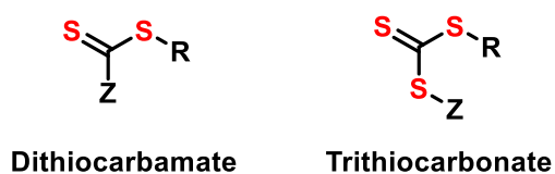
Figure I-4 General structure of CTAs used in RAFT polymerization.
