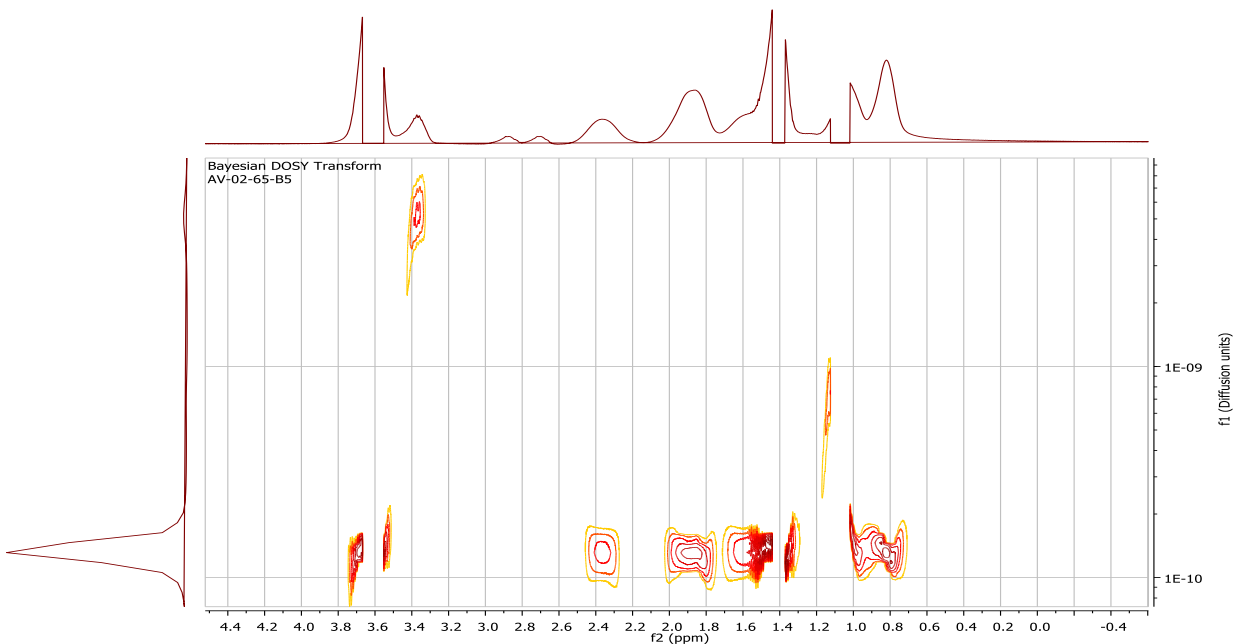
Figure II-17 DOSY spectra of MMA 280 AA 100 . \Delta = 0.2 s; \delta = 2 ms; g was varied from 27 mT/m to 0.27 T/m.
