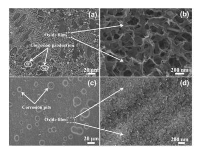
**Figure 5.** Corrosion morphologies of Al-12Si after 14 days immersion in 3.5 wt. % NaCl solution: (**a**,**b**) as-casted Al-12Si alloy; (**c**,**d**) SLM produced Al-12Si alloy [64].
