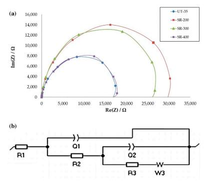
**Figure 12.** EIS spectra of the samples tested in Harrison solution: (**a**) Nyquist plot; (**b**) the fitting equivalent circuit [83].
