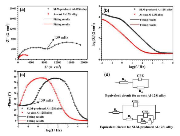
**Figure 9.** The EIS plots of SLM and casted Al-12Si aluminum alloy: (**a**) Nyquist plots; (**b**,**c**) Bode plots; (**d**) fitting equivalent circuit diagram [65].
