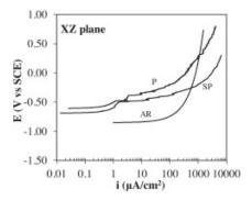
**Figure 8.** Polarization curves of printed AlSi10Mg alloy in diluted Harrison's solution on XY specimens with different surface treatment [91].
