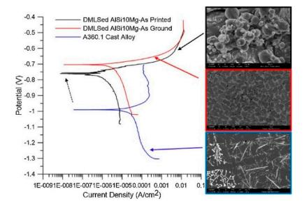
**Figure 6.** The polarization curves of printed, ground and casted aluminum alloy produced by DMLS [90].
