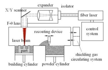
Figure 1. The schematic diagram of SLM [28].
