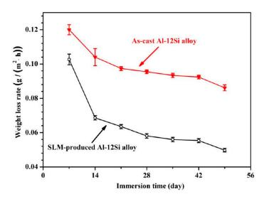
**Figure 4.** Weight loss rate of the SLM produced Al-12Si and casted Al-12Si after immersion in the aerated 3.5 wt. % NaCl solution [64].
