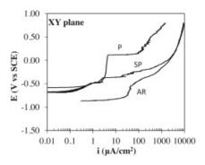
**Figure 7.** Polarization curves of printed AlSi10Mg alloy in diluted Harrison's solution on XY specimens with different surface treatment [91].
