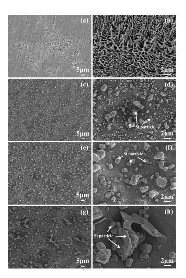
**Figure 11.** SEM micrographs of SLM produced AlSi10Mg alloys after 45 days immersion in 3.5 wt. % NaCl solution: (**a**,**b**) untreated; (**c**,**d**) post heat treatment at 450 °C; (**e**,**f**) post heat treatment at 500 °C; (**g**,**h**) post heat treatment at 550 °C [67].
