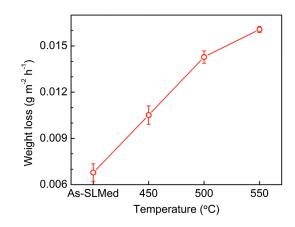
Figure 10. Weight loss of untreated and additionally heat-treated SLM AlSi10Mg alloy [67].
