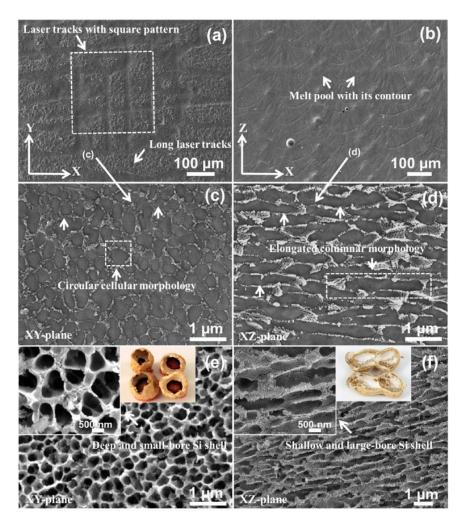
**Figure 2.** The microstructure of two different planes of SLM Al-12Si alloy: (**a**) polished XY plane; (**b**) polished XZ plane; (**c**) eutectic Si networks of XY plane; (**d**) eutectic Si networks of XZ plane; (**e**) the eutectic Si shells of XY plane; (**f**) the eutectic Si shells of XZ plane [68].
