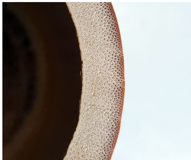
Figure 1 Cross section of bamboo culm showing a non-uniform distribution of fibres through the thickness.
