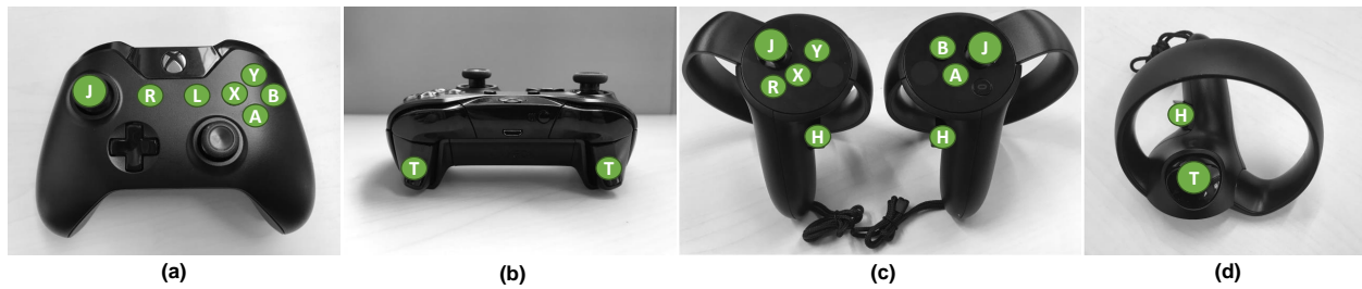
Figure 3. Various VR controllers : (a–b) an Xbox gamepad controller; (c–d) Oculus Touch. The green markers with accompanying letters are showing mapping between the action-buttons on both types of controllers. The description of user’s movement in the 3D space together with interaction details can be found in Tadeja et al. 5,6
