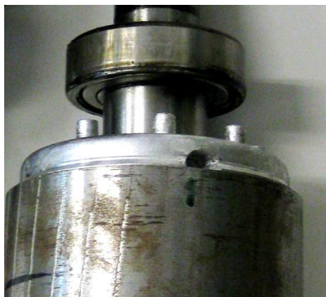
Fig. 1. Rotor bar drilled at one of its ends.
