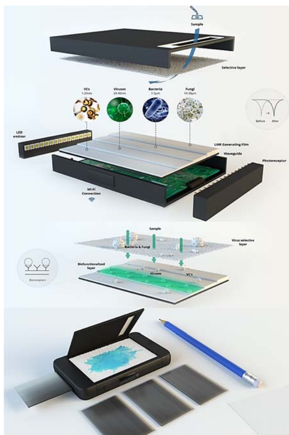
Fig. 1. Setup of the label-free multipurpose sensor. At the top, a schematic of the sensing platform. In the middle, a practical application of the platform towards detection of a type of virus. At the bottom, an infographic of the final device with the detection cartridges.
