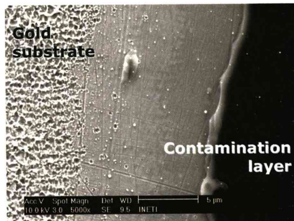
Fig. 61 . Laser inhomogeneous cleaned areas
