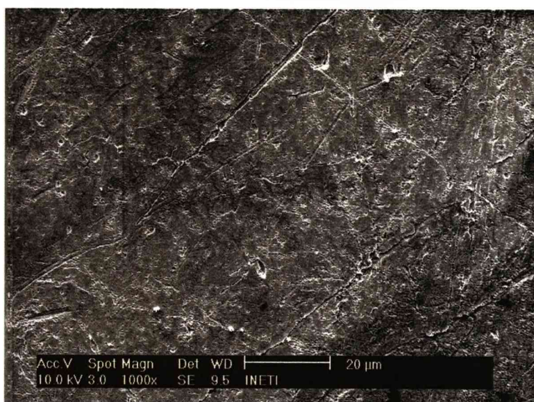
Fig. 57. Bare gold surface (GM02) single scanned E = 2 \mu\text{J} , OS = 1, spot diameter = 25 \mu\text{m}
