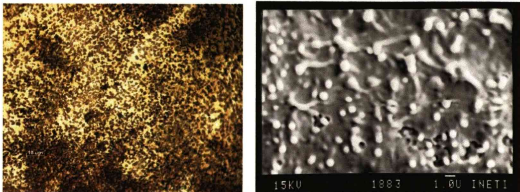
Fig. 32. The Year of the Horse Coin (YHC06) showing modifications on the surface, after irradiation with 0.37 \text{ J cm}^{-2}
