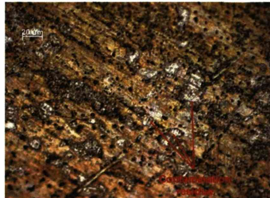
b) under cleaned surface, band I ( F=30 \text{ mJ cm}^{-2} OL=5, OS=4)
