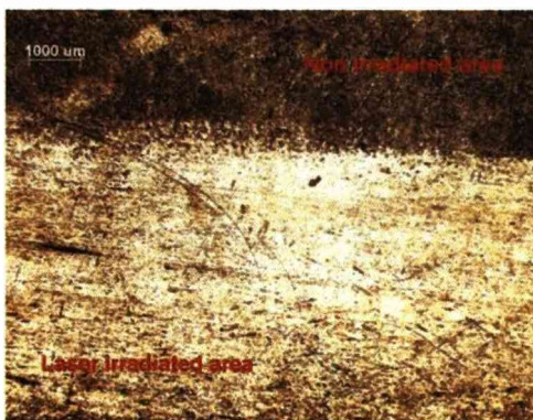
c) cleaned area band II X10 (left), x2500 (right) ( F=60 \text{ mJ cm}^{-2} , OL=5, OS=2)
