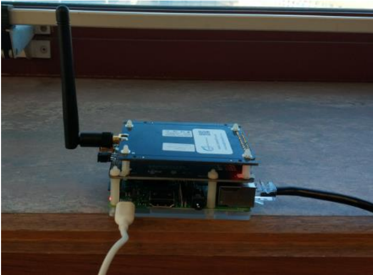
Fig.4- 5 The LoRaWAN gateway.
