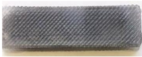
Figure 5-2 Sample geometry of fused filament fabricated PLLA-SS420 composites
