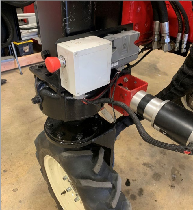
Figure 2.13: One of four red e-Stop buttons located on exterior of machine for quick and safe access.
