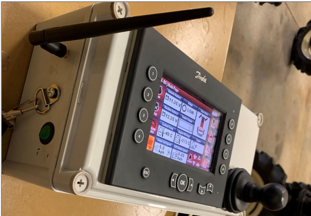
Figure 2.1: Remote control box developed for teleoperation of the Flex-Ro platform.
