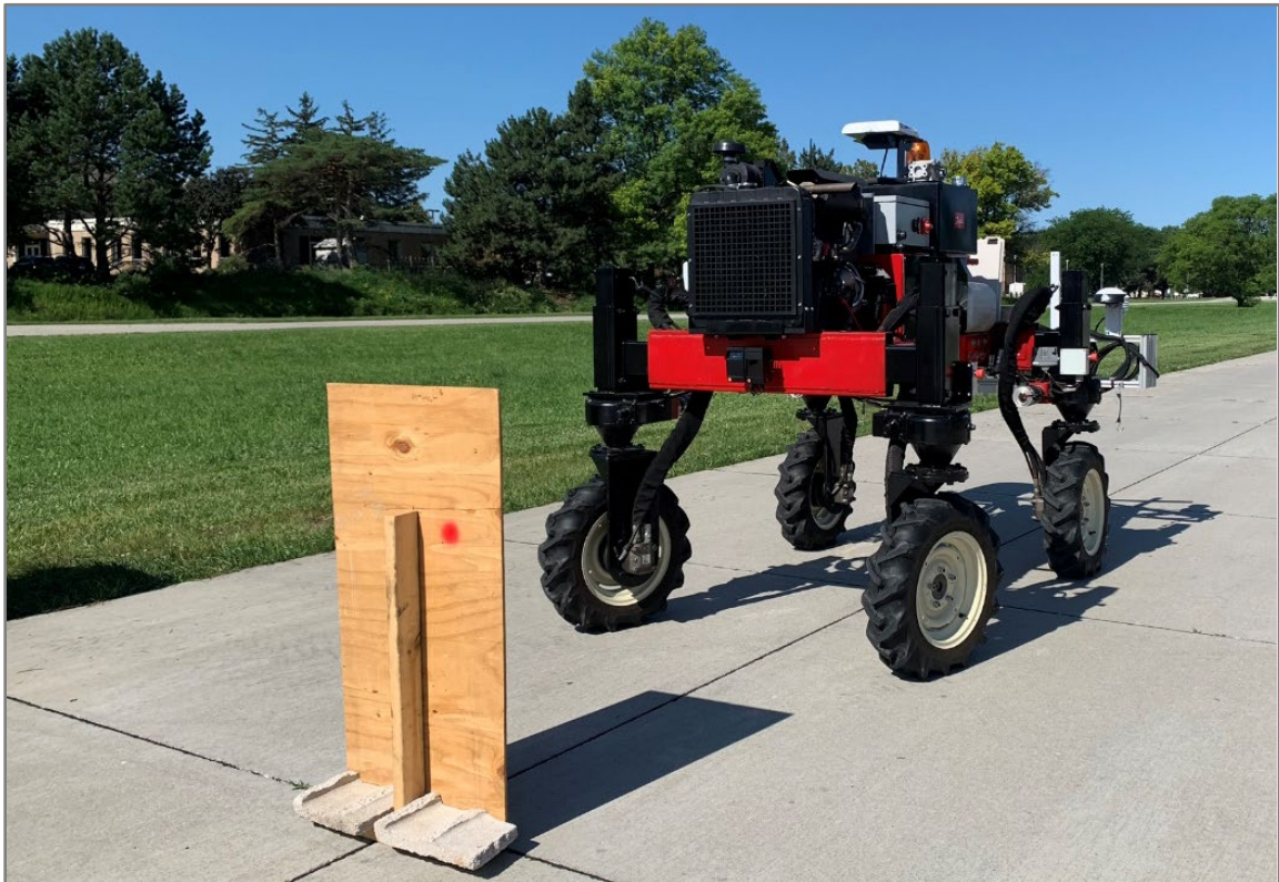
Figure 2.19: Dynamic obstacle approach test. Stopping distance was measured from detector on front to board.
