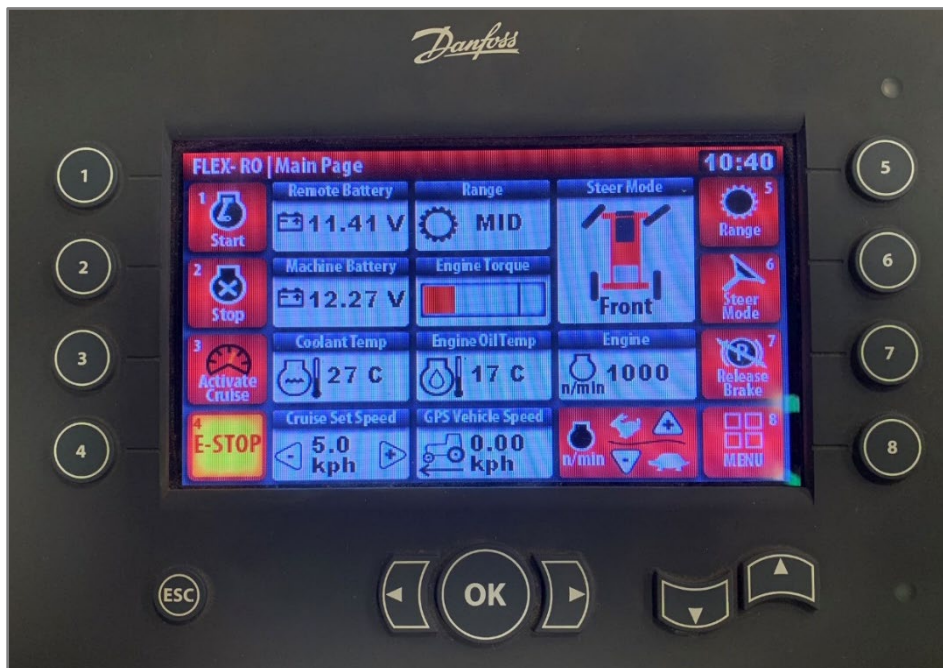
Figure 2.3: Main operating screen of the Flex-Ro remote. Danfoss DP600TM display.
