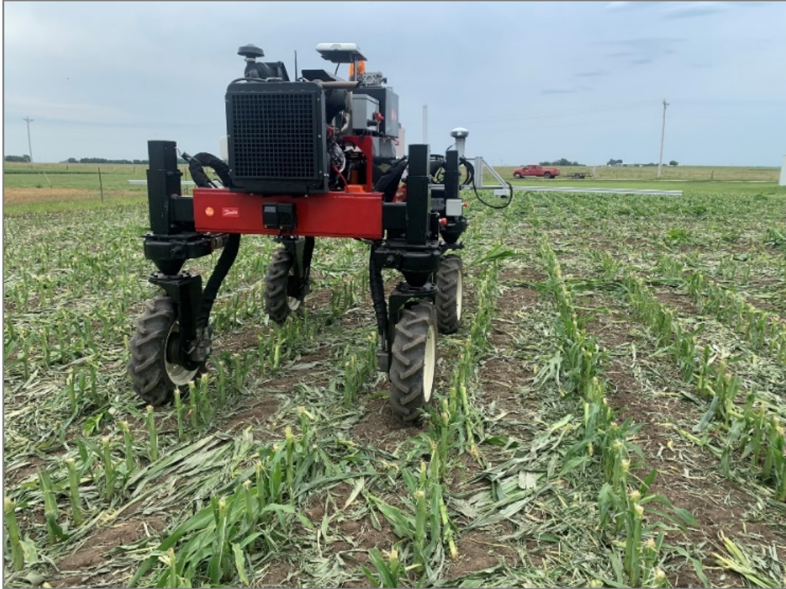
Figure 2.14: Testing AB line navigation in corn stubble.
