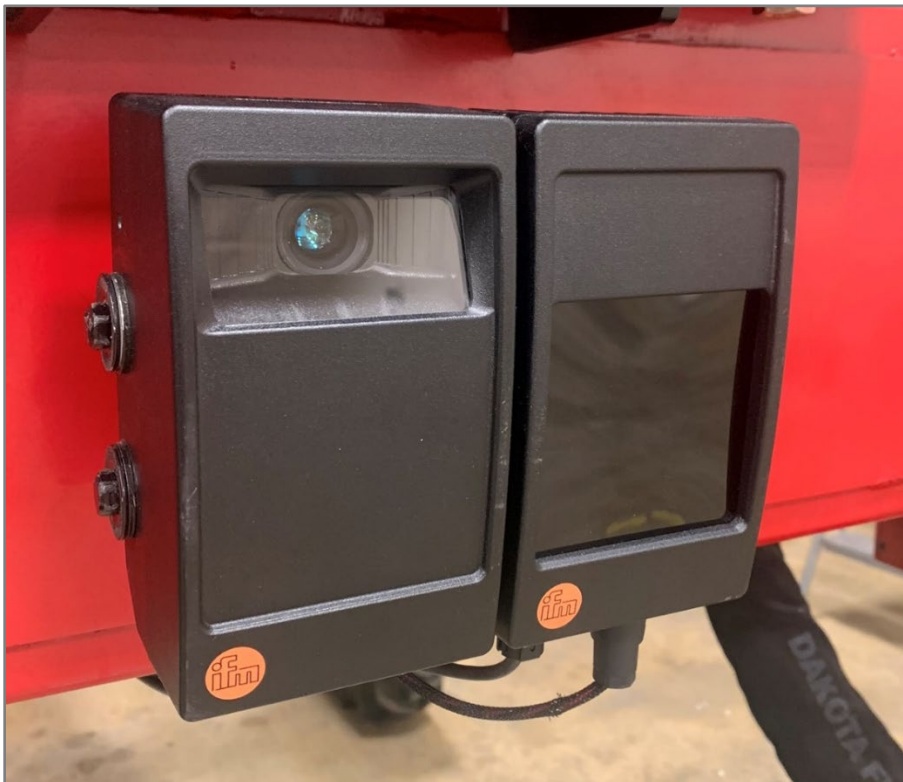
Figure 2.11: ifm O3M 151 3D Smart Sensor installed on the front of the Flex-Ro platform.
