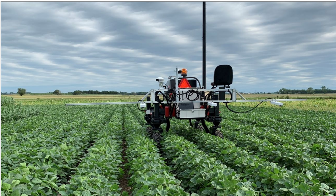
Figure 3.6: The Flex-Ro collecting data 67 days after planting (DAP). Each of the sensor units are positioned directly over a row.
