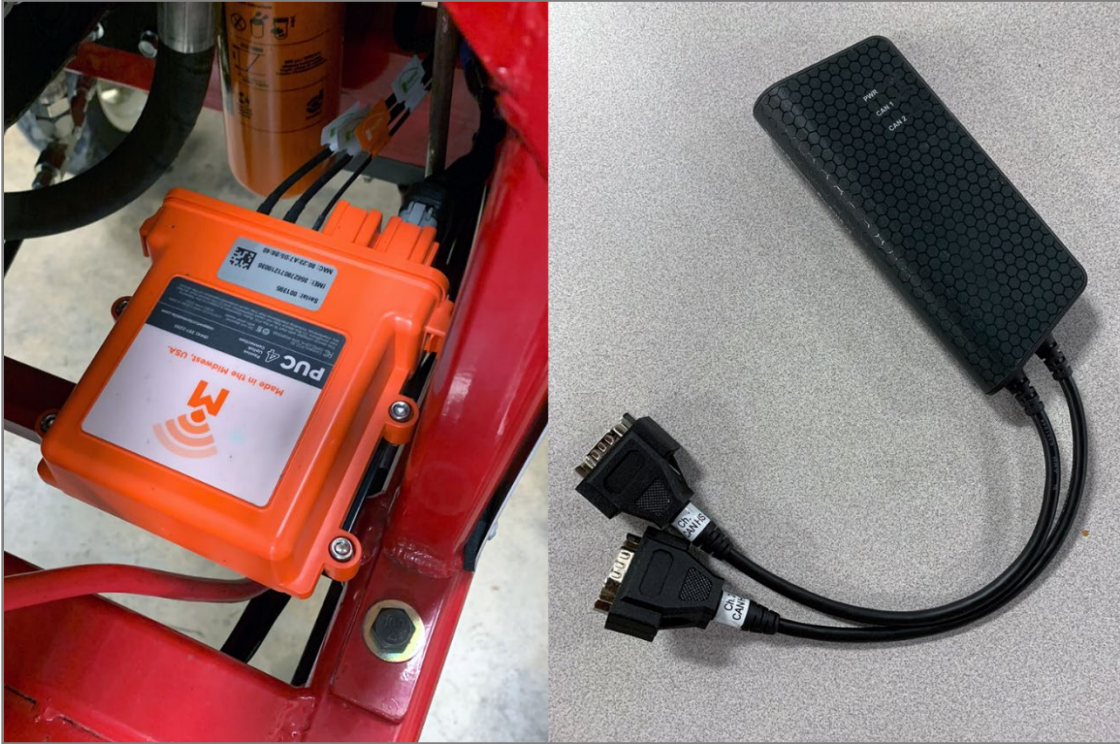
Figure 4.1: Left: Farmobile PUC data streaming device. Right: Kvaser Memorator Pro 2xHS v2 CAN logger.
