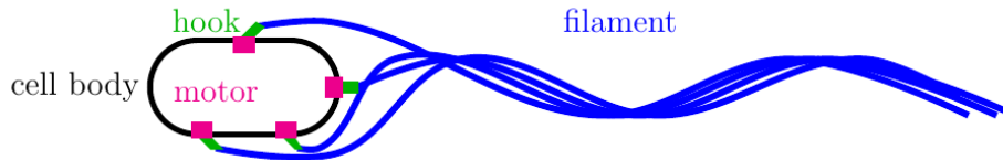
Figure 5.1: A cell body with four flagella. When each flagella's motor spins counter-clockwise, the flagella combine to form a superflagellum which propels the cell forward. This image is reproduced from Ko et al. [1].
