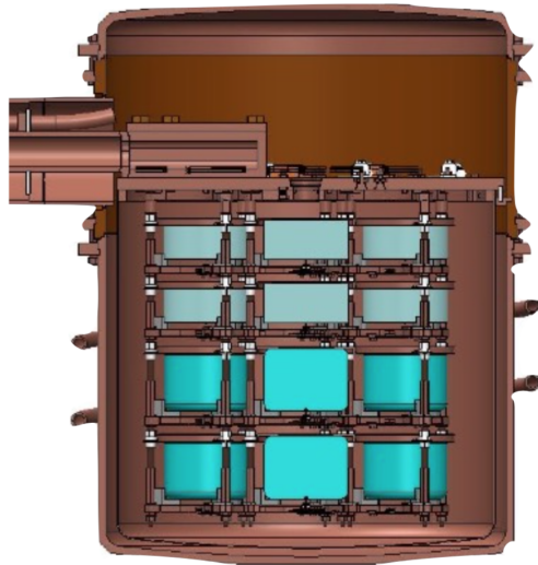
Figure 3.1: A cross sectional rendering of one MJD cryostat containing an array of detectors (teal and grayish-teal). The detectors are stacked vertically into strings prior to installation in a cryostat. Enriched detectors occupy the bottom two rows of each string in this rendering, with natural detectors occupying the top two rows.
