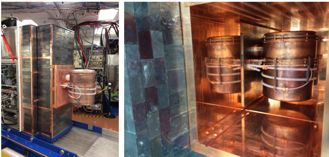
Figure 7.5: PTFE tubing wraps helically around each cryostat forming a track for a calibration line source.
