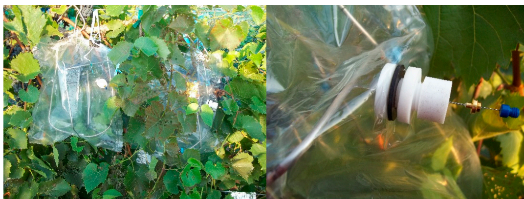
Figure 2. Biogenic volatiles were collected with SPME using an enclosure made from a polyvinyl fluoride (PVF) film to temporarily envelop a whole growing cluster of grapes ( left ). SPME is inserted into enclosure via a sampling port ( right ).
