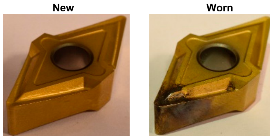
Figure 11. Visual representation of the new cutting tip (left) and worn cutting tip (right) used for the lathe tool wear investigation.
