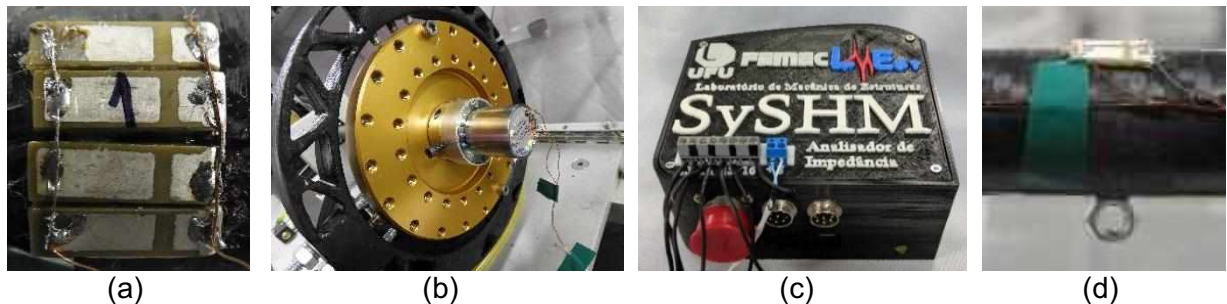
Figure 5.3 - (a) Piezoelectric transducer; (b) Slip ring attached to the disc-2; (c) Impedance measurement system, (d) Nut bonded on the composite shaft to simulate damage.
