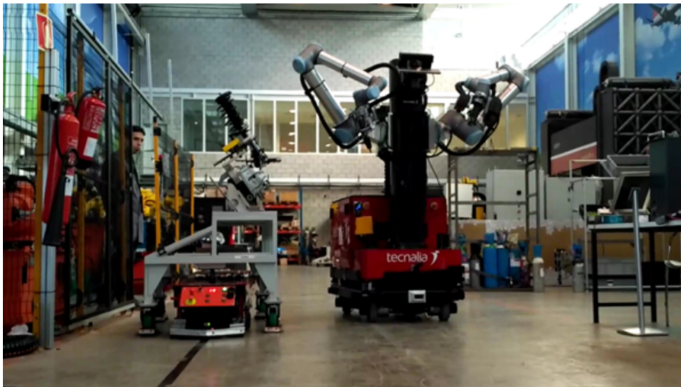
Figure 13. MRP following the mobile product platform (MPP) through the dynamic docking (visual servoing) system.
