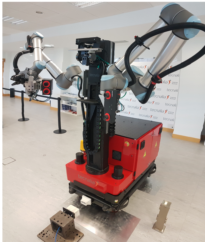
Figure 1. The Mobile Robotic Platform (MRP) navigating autonomously to the charging station.
