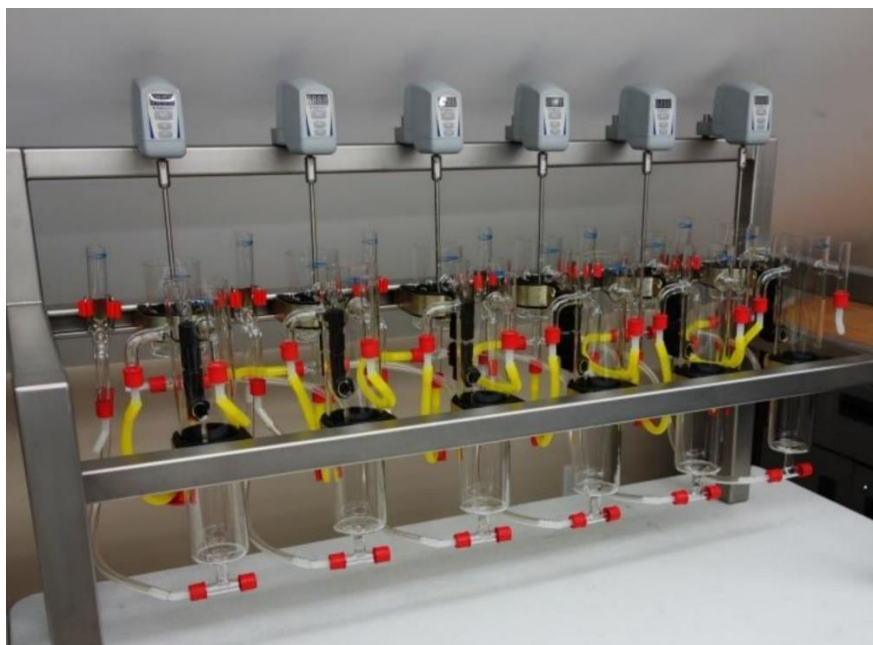
Figure 3.13 Laboratory scale setup of the solvent extraction equipment comprised of six glass mixer settlers used for continuous testing of the solvent extraction circuit.
