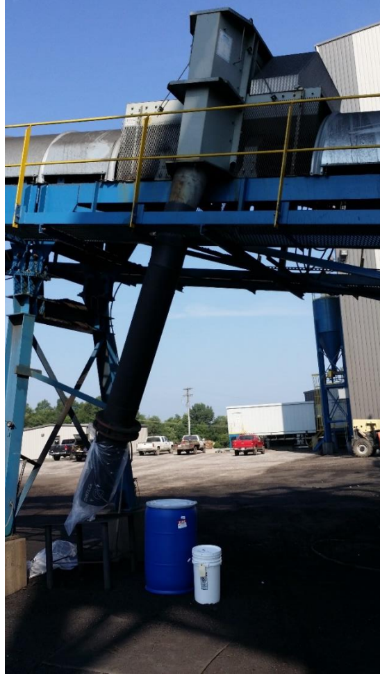
Figure 3.4 Sweep-belt sampler used to collect representative samples from the coarse refuse process stream of a coal preparation plant.
