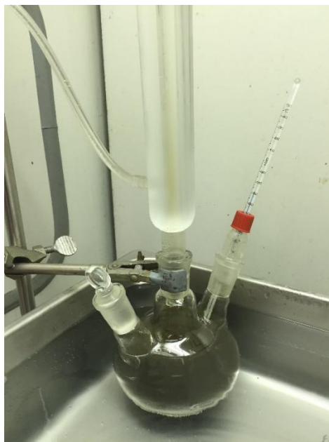
Figure 3.8 Experimental setup used for leaching tests in the study.
