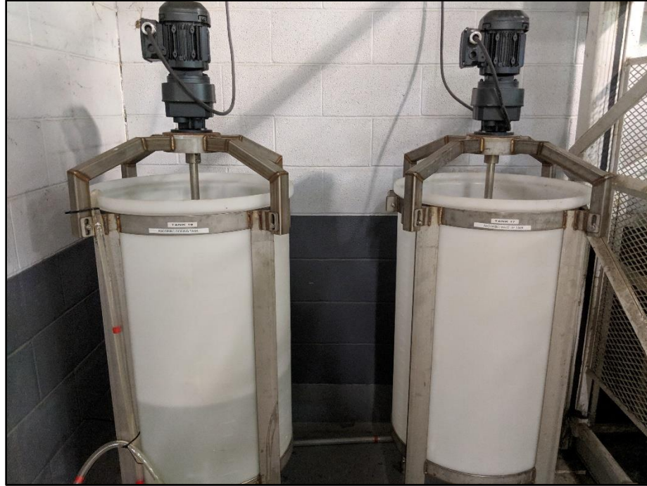
Figure 4.22 Tanks used for mixing and dosing the ascorbic acid to the feed solution for the solvent extraction process.
