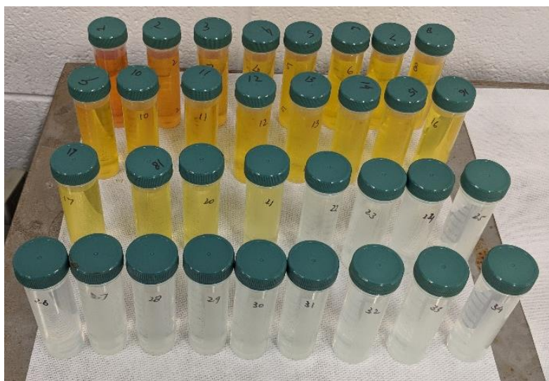
Figure 4.1 Visual change in the color of the test solution with incremental additions of 200g/L (1.136 M) solution of ascorbic acid.
