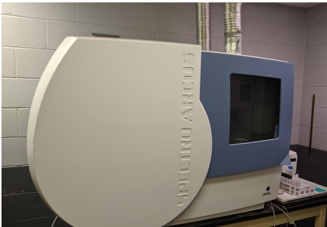
Figure 3.14 Inductively coupled plasma - optical emission spectroscopy (ICP-OES) apparatus at the University of Kentucky used for elemental characterization of the aqueous phase.
