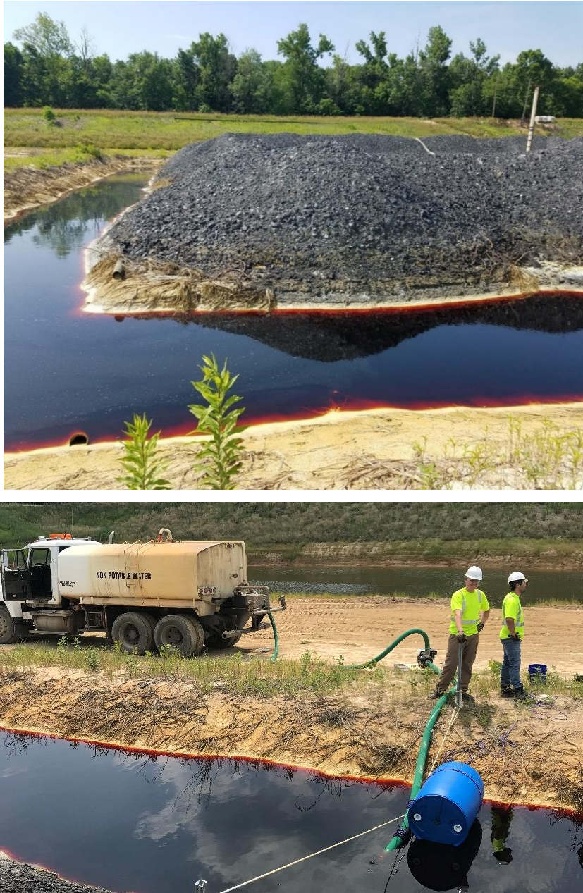
Figure 3.6 The site for generation of heap leachate from the coal coarse refuse of Dotiki coal preparation plant.
