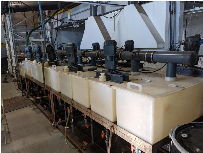
Figure 3.11 Conventional mixer-settler setup used in the pilot-scale continuous scale solvent extraction testing.
