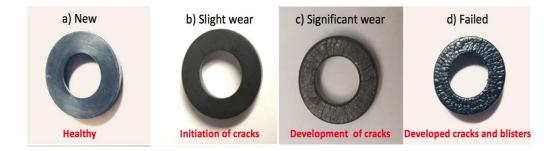
Figure 11: Development of Aging Signs in Rotary Seals During Aging
