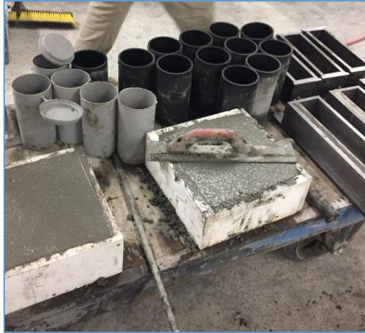
(b) Molds being finished
