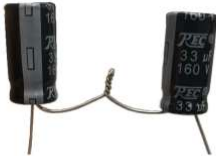
Figure 7. Single-phase AC capacitor.
