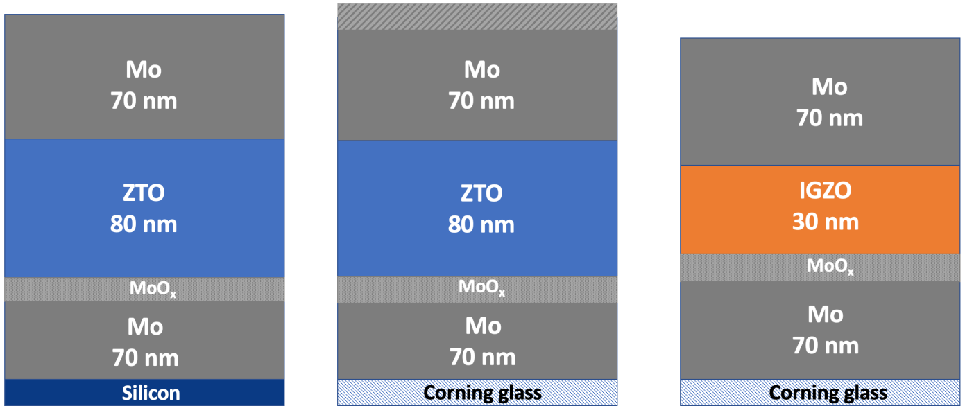
Figure 7.1 – Cross section for the three types of samples produced. The first Mo/ZTO/Mo device had its bottom molybdenum contact oxidized upon the deposition of the ZTO layer on the sputtering chamber whereas the other two devices (ZTO passivated and IGZO) had their bottom contact oxidized via an oxygen plasma treatment.
