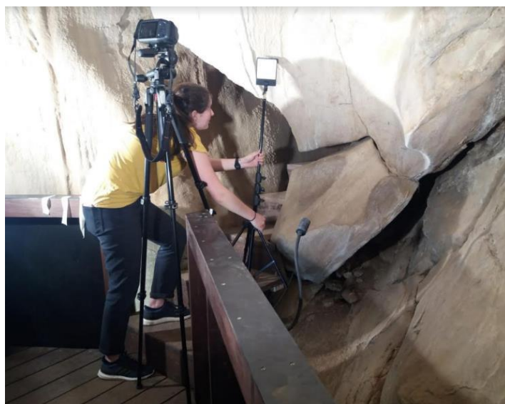
Hyperspectral camera being set up at Escoural Cave; painting #2. Lighting and white reference are being adjusted for optimal conditions.
