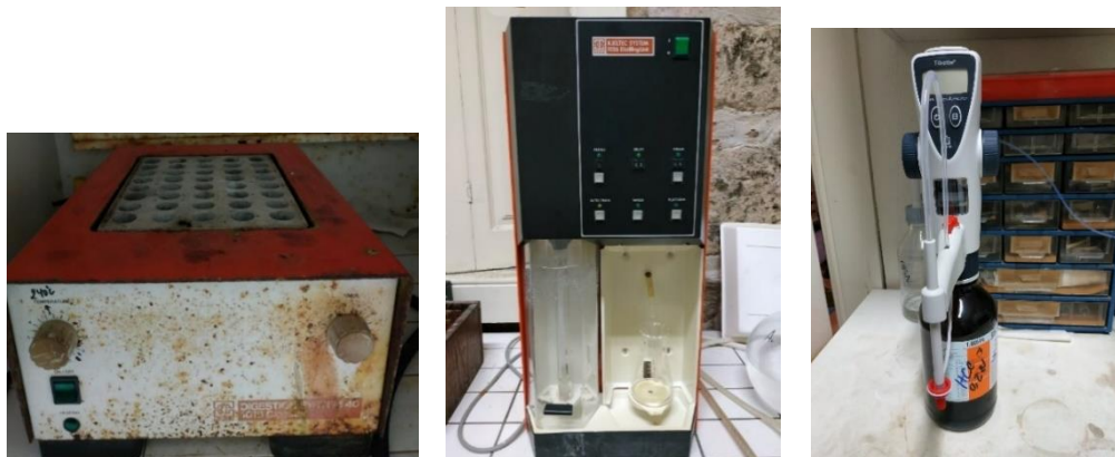
Figure 24: At the left: a Kjeldahl digestion unit; In the middle: a distillation unit; At the right: a titration unit.
