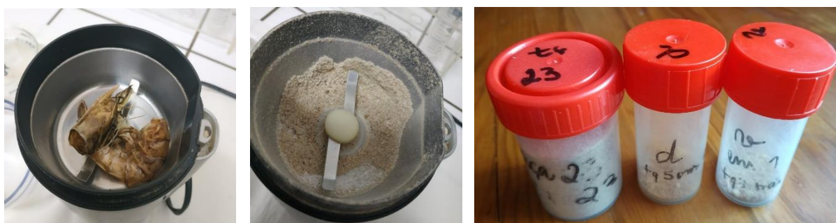
Figure 23: At the left: dry shrimp in a coffee grinder; In the middle: powdered shrimp; At the right: identified falcons containing powdered shrimp.
