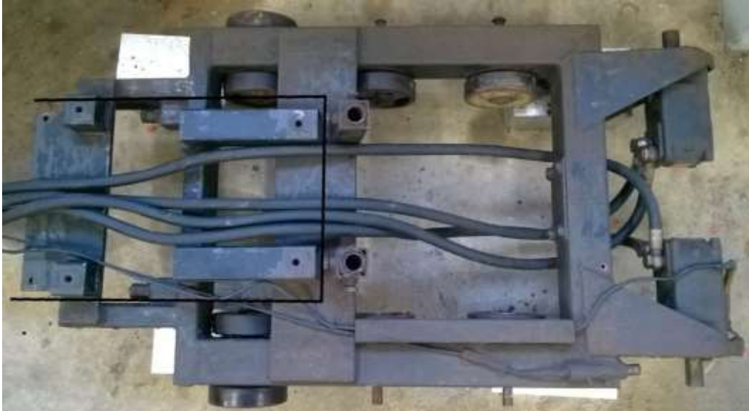
Figure 5.31 – Frame modification cutting lines
