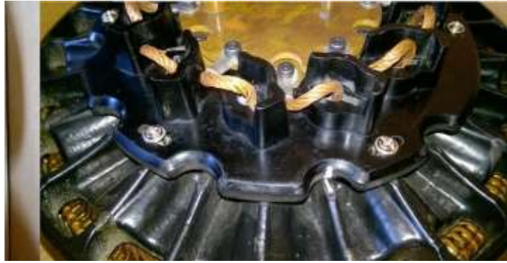
Figure 5.57 – Detail of Agni 155R motor with replaced brush holder
