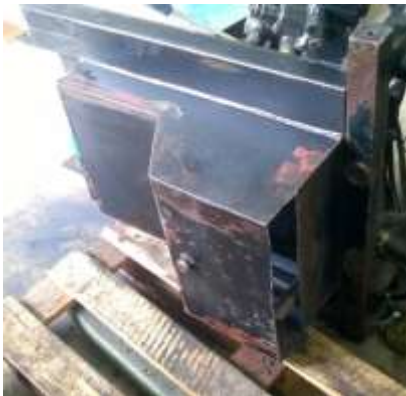
Figure 5.36 – Oil reservoir rear cut
