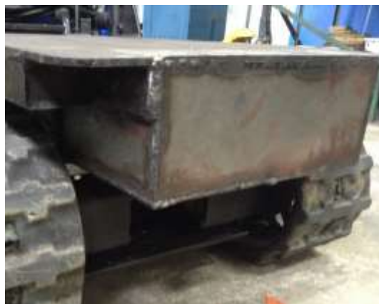
Figure 5.39 – Oil reservoir front view after change, right view
