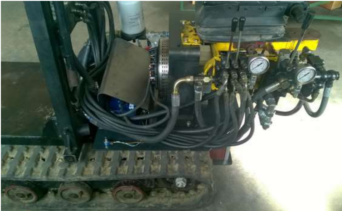
Figure 5.70 – Final look of prototype, detail of electric motor, batteries and controller
