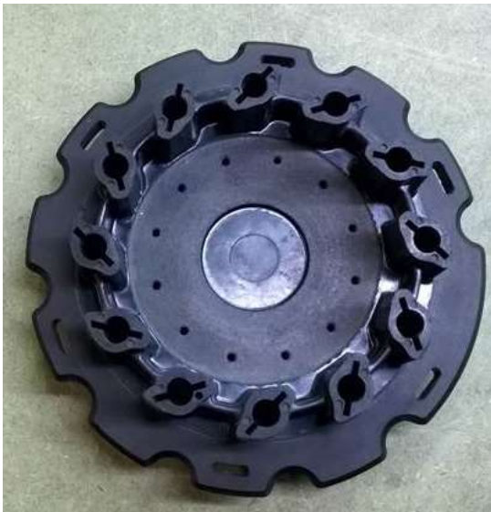
Figure 5.54 – New brush holder, inside view
