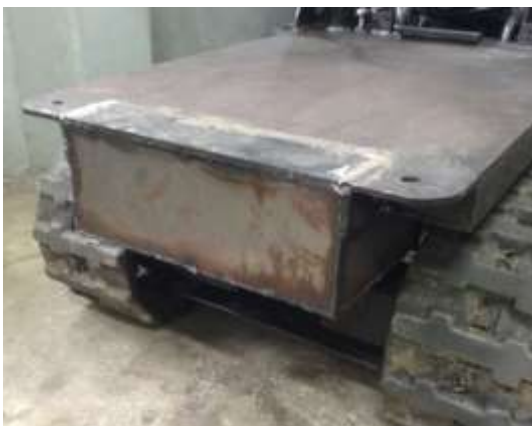
Figure 5.38 – Oil reservoir front view after change, left view
