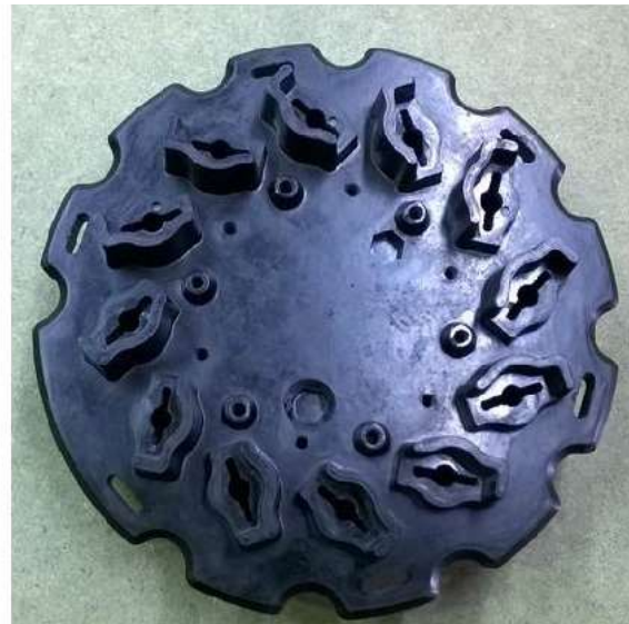
Figure 5.55 – New brush holder, outside view
