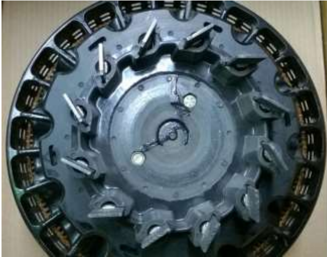
Figure 5.52 – Brush holder center cracked
