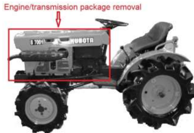
Figure 4.02 – Placement of engine/transmission in a small tractor
