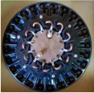
Figure 5.56 – Agni 155R motor with replaced brush holder
