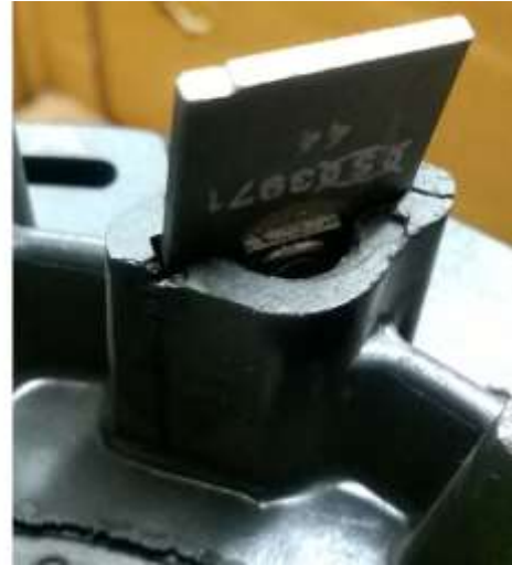
Figure 5.53 – Individual brush holder with cracks
