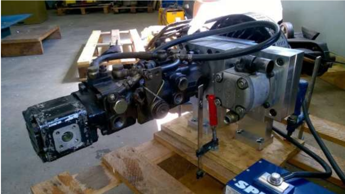
Figure 5.64 – Transmission box first test, May 2015
