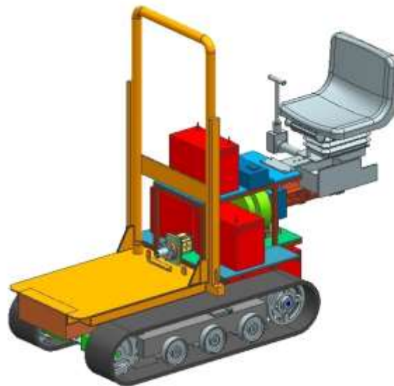
Figure 5.29 – Six batteries solution, version 2 isometric view
