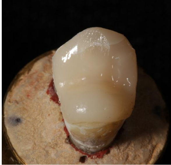
Fig. 18. Specimen showing some cracks after thermomechanical loading (partial success)
