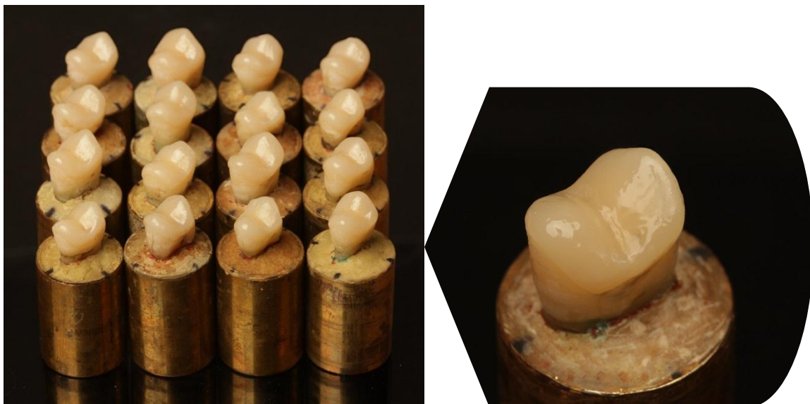
Fig. 16. Specimens after adhesive luting in group LD
