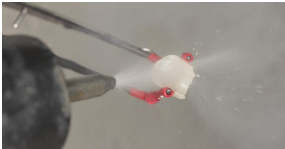
Fig. 10. Water steam cleaning of a milled occlusal veneer
