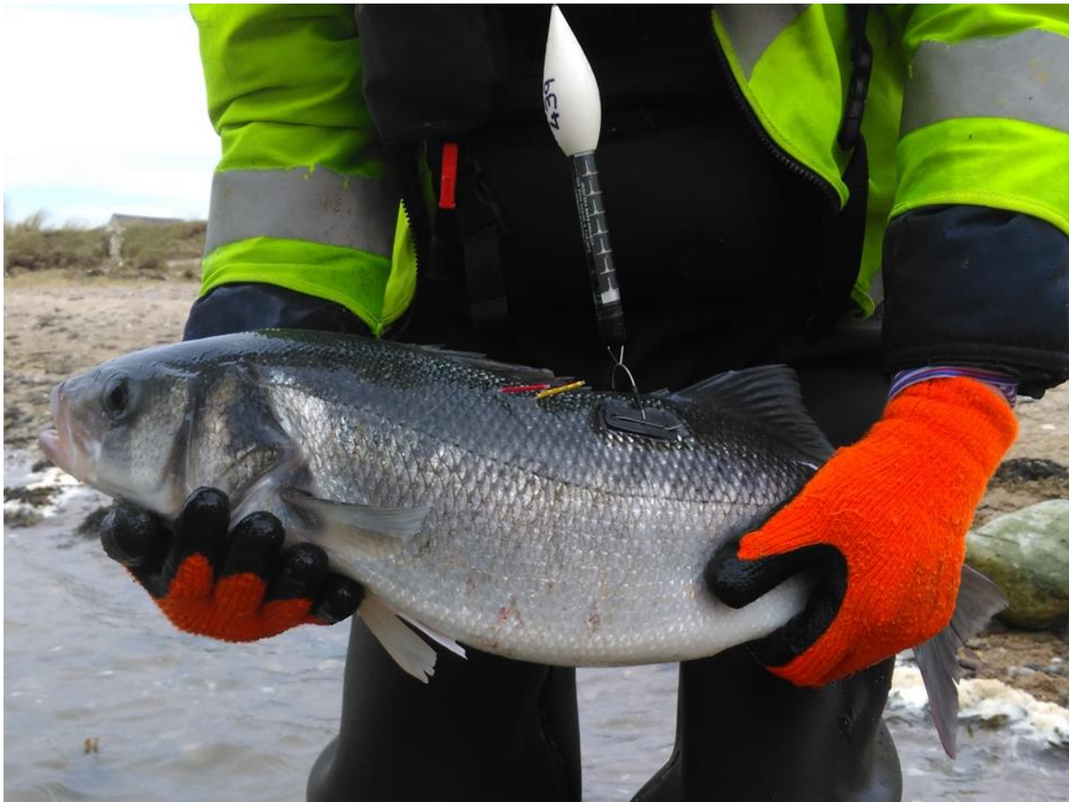
Fig. 1. Dicentrarchus labrax fitted with a Desert Star Systems SeaTag-GEO pop-up satellite tag (PSAT) and corresponding tag bridle with additional Floy tags for identification.
