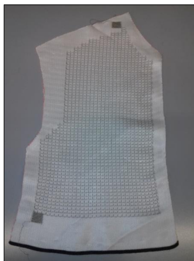
Figure 2: Knitted cut sensor (left front side of cardigan)
