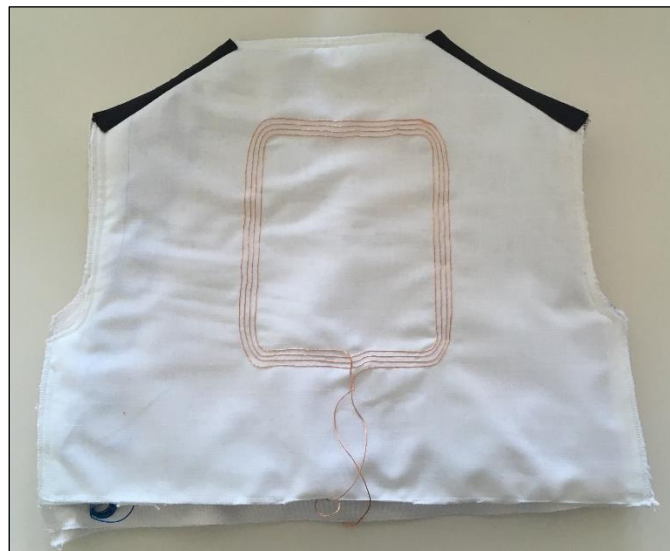
Figure 6: Tailored jacket inlay with induction coil and Velcro® strips for fastening
