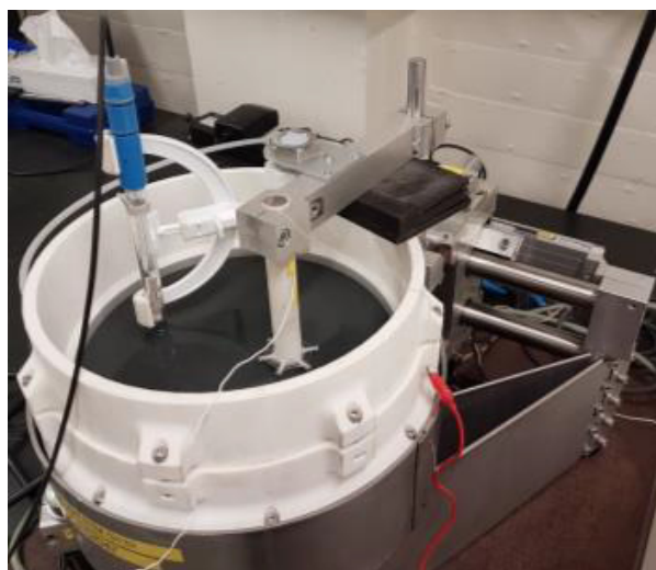
Figure 1: Two-body abrasion-corrosion tester coupling
