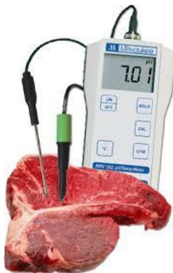
Figure A.10 A pH meter measuring the pH of beef steak muscle. A pH probe is inserted approx. 1 cm into the flesh and a measurement taken.
