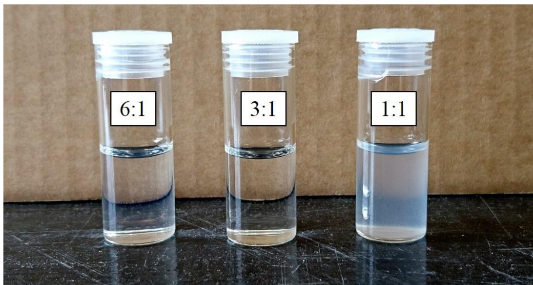
Figure 2.2 Visual Image of chitosan nanoparticle synthesised from 0.1 % low molecular weight chitosan at pH 4.6 using 6:1, 3:1 and 1:1 CS:TPP mass ratios (from left to right) where 1:1 is the most turbid while 3:1 is least turbid.
