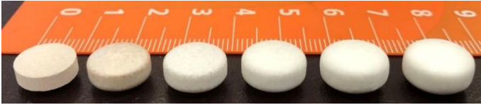
Fig. 1. Photographs of uncoated cores and HPMC-coated systems having increasing coating level (ruler scale in cm).
