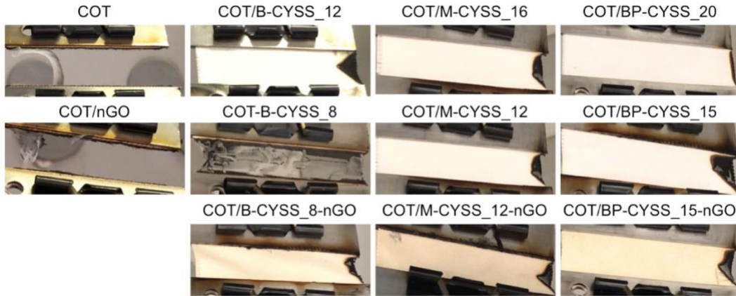
Figure 8. Snapshots of untreated, SS-PAA, nGO- and SS-PAA-nGO treated cotton in horizontal flame spread tests.
