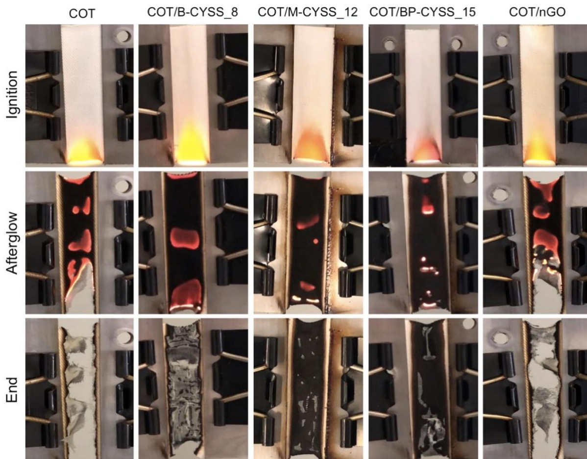
Figure 6. Snapshots of untreated, SS-PAA- and nGO treated cotton in vertical flame spread tests.
